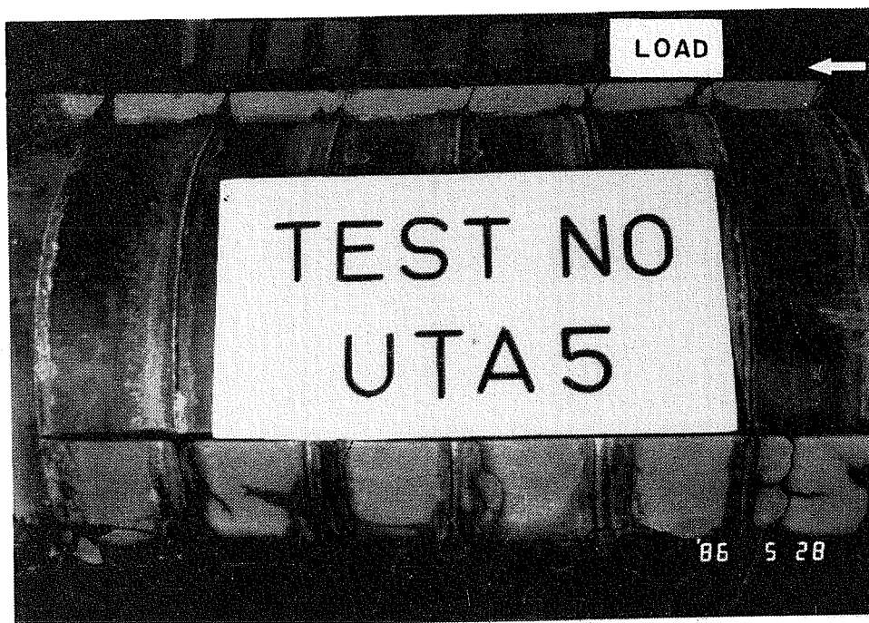
Fig. 3.10 Grout profile of Specimen UTA5 showing crack pattern
