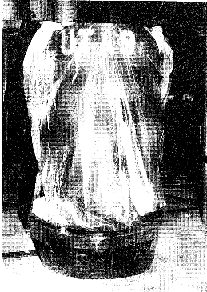
Fig. 2.12 Typical specimen storage during curing
